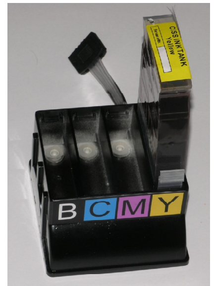
Place reservoir cartridge into position that matches color and type
